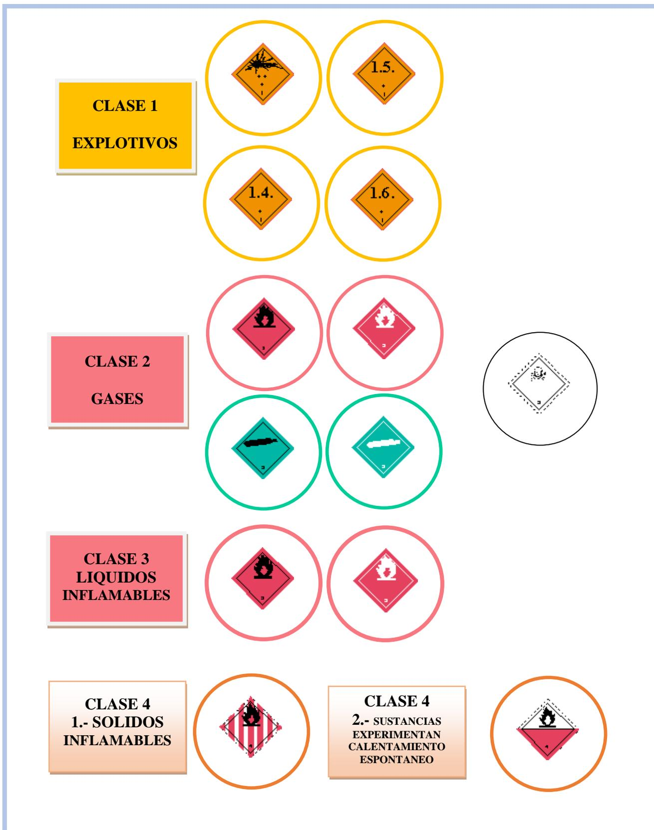
The diagram illustrates the classification of dangerous goods into five classes, each with a corresponding color-coded box and hazard pictograms:
